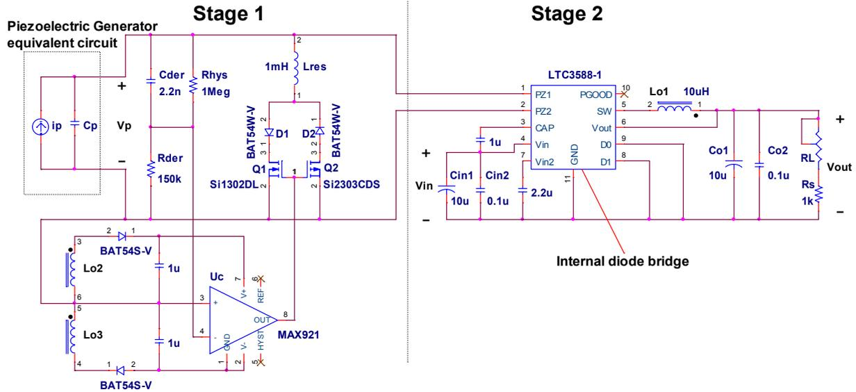
Fig. 5. Proposed self powered resonant rectifier circuitry with auxiliary windings and regulated output voltage.
