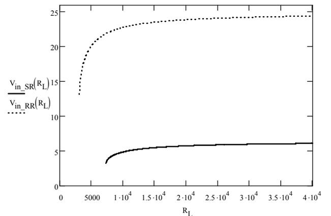
Fig. 2. Analytical comparison between average output voltages ( $V_{in}$  of converter) of the resonant rectifier interface and the standard interface versus output load  $R_L$ .
