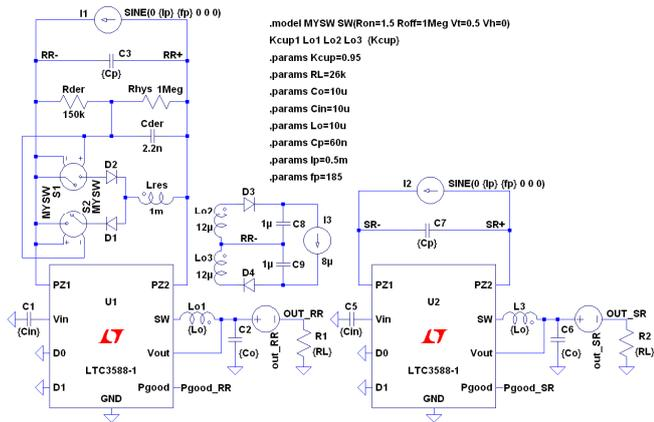
Fig. 3. Simulation diagram of the standard rectifier (right side) and the resonant rectifier (left side). The auxiliary windings ( $L_{o2}$  and  $L_{o3}$ ) are coupled to the main DC inductor ( $L_{o1}$ ) and used to feed the comparator by an approximately constant voltage. The average current drawn from the power supplies of the comparator (8 $\mu$ A) is an overestimated current consumption of the comparator.
