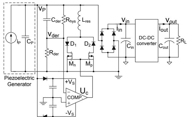
Fig. 1. A resonant rectifier interface connected to a DC-DC converter. The input voltage of the circuit is limited by the maximum ratings of the comparator's power supplies.
