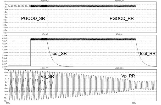
Fig. 4. Simulation waveforms of 1.8mA load step response of the two configurations. See Fig. 3 for notations.
