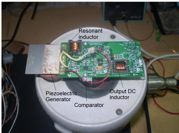
Fig. 6. Experimental setup and circuit prototype. Piezoelectric generator (with free end) is clamped to a PCB. The whole system is mounted on a shaker that provides vertical (z-axis) sinusoidal vibration.
