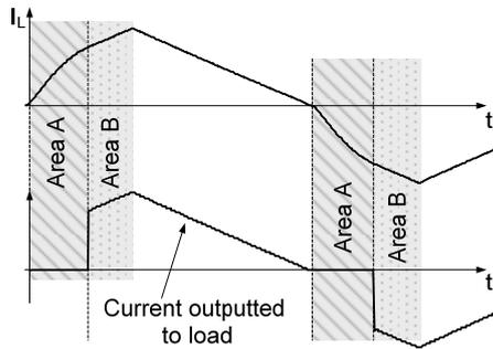
Figure 14. Effect of parasitic capacitance. Large capacitance.
