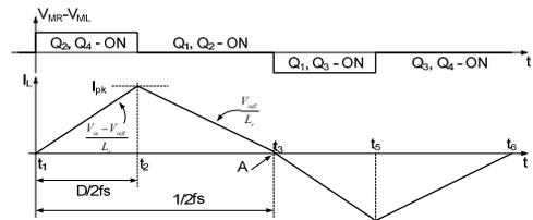
Figure 3. Inductor current of an isolated TCS converter operating under ZCS and ZVS at turn-on.
