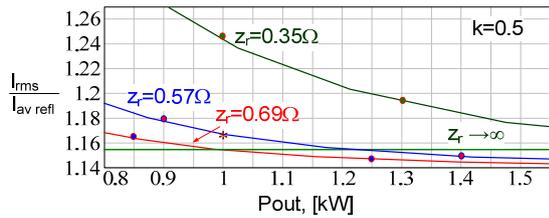
Figure 7. Ratio of input rms current to output average current reflected to the primary for different parasitic capacitors and primary-to-input voltage ratio ( $k$ ) 0.5.  $V_{in}=24V$ . Solid line: theoretical predictions; Dots: cycle-by-cycle simulation results. Asterisk : Experimental converter
