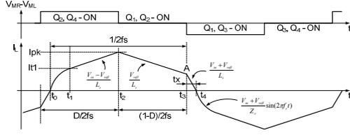
Figure 4. Inductor current of an isolated TCS converter with parasitic capacitance.
