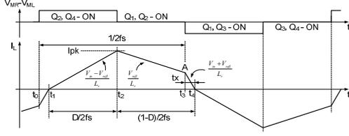
Figure 2. Inductor current of an isolated TCS converter.
