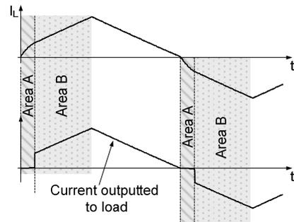
Figure 13. Effect of parasitic capacitance. Small capacitance.
