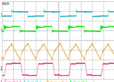
Figure 12. Experimental results.  $C_{\text{sec}} \approx 160\text{pF}$ .
