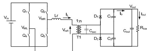
Figure 1. Isolated TCS converter with voltage doubler at the output side.
