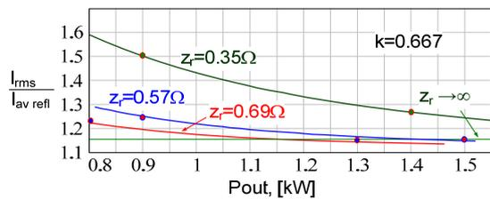
Figure 8. Ratio of input rms current to output average current reflected to the primary for different parasitic capacitors and primary-to-input voltage ratio ( $k$ ) 0.667.  $V_{in}=24V$ . Solid line: theoretical predictions; Dots: cycle-by-cycle simulation results.
