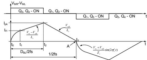
Figure 5. Inductor current of an isolated TCS converter operating in BCM (with parasitic capacitance).
