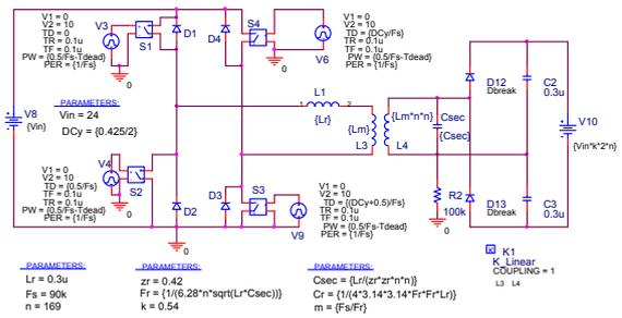
Figure 9. PSPICE cycle-by-cycle simulation model.
