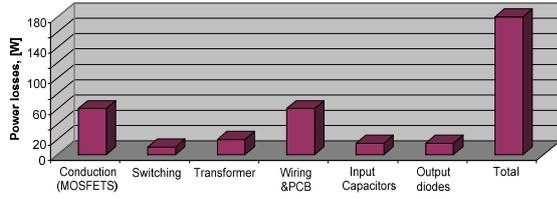
Figure 11. Estimated power losses distribution of experimental breadboard.
