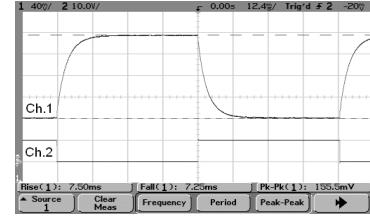
Fig. 12. Response to load ( $R_o$ ) change from  $3.6k\Omega$  to  $128 \Omega$ .  $V_{in} = 8V$ ,  $M_3 = 3/8$ . Vertical scale: 40mV/div; Horizontal scale: 12.4ms/div. Ch.1: output voltage, Ch.2: load step control signal. Peak to peak output voltage change is 155.5 mV.
