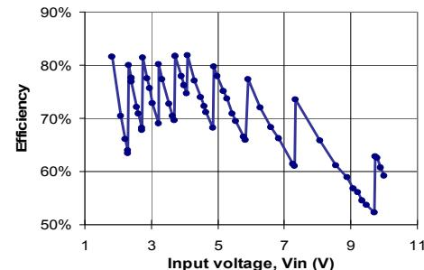
Fig. 16. Efficiency of EXB based SCC operating with an LDO at the output in both step-down and step-up modes.  $V_o$  set to 3.3V
