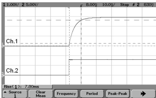
Fig. 11. Output voltage from start up.  $V_{in} = 8V$ ,  $M_3 = 3/8$ , Load resistor  $R_o = 3.6k\Omega$ . Vertical scale: 1V/div; Horizontal scale: 10ms/div.
