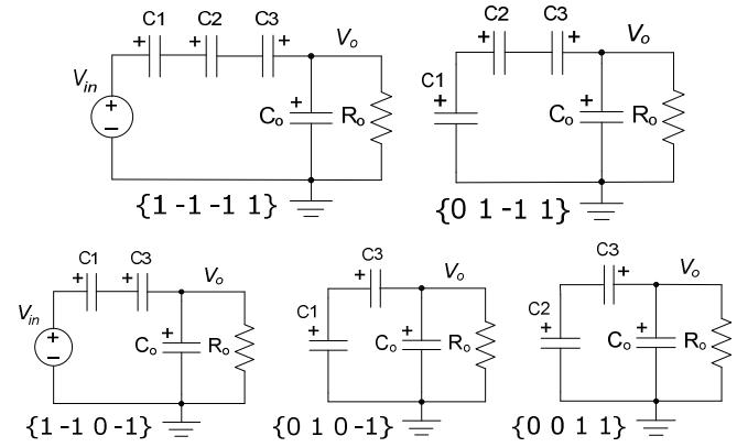
Fig. 4. Capacitors connections that follow the EXB codes of  $M_3 = 3/8$ .
