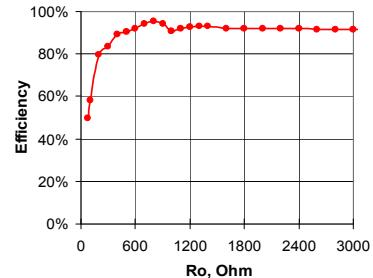
Fig. 15. Efficiency of step-up EXB based SCC,  $M_3 = 8/3$ .
