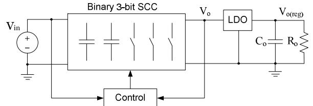
Fig. 9. Block diagram of output voltage regulation by LDO at the output.
