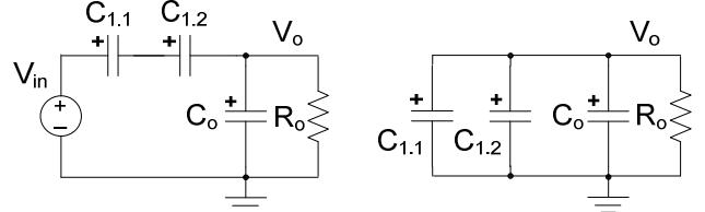
Fig. 5. Capacitors connections that follow the GFN codes of  $N_1(3) = 1/3$ .
