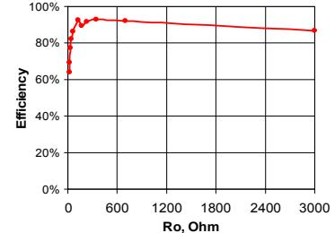
Fig. 14. Efficiency of step-down EXB based SCC,  $M_3 = 3/8$ .
