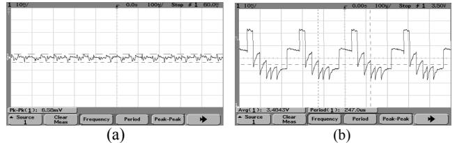
Fig. 13. Output ripple.  $V_{in}=8V$  and  $R_o = 437 \Omega$ . (a)  $M_3 = 3/8$ . (b) Dithering between  $M_3 = 3/8$  and  $M_1 = 1/2$  (in 4:1 ratio). Vertical scale: 10mV/div; Horizontal scale:  $100\mu S$ /div.
