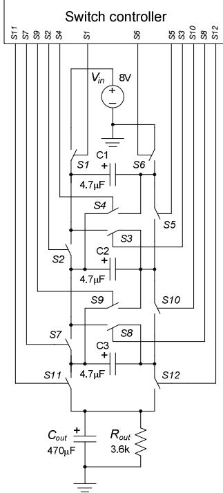
Fig. 10. Interconnection of switches and capacitors of the proposed binary SCC for  $n=3$  as used in experimental setup
