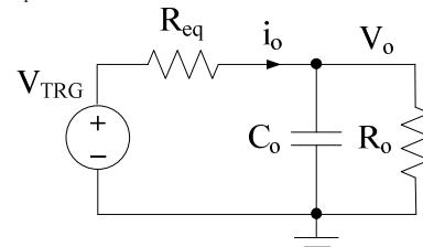
Fig. 2. The SCC equivalent circuit.
