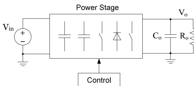
Fig. 1. The switched capacitor converter (SCC) concept.
