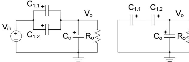
Fig. 6. Capacitors connections that follow the GFN codes of  $N_1(3) = 2/3$ .
