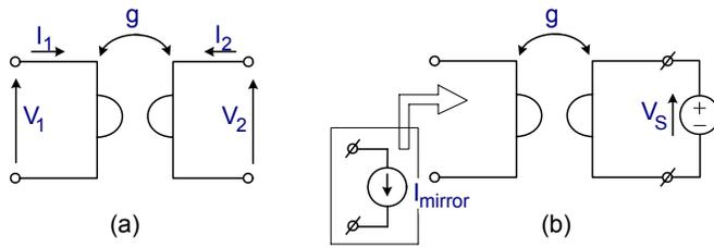
Figure 1: (a) Gyrator symbolic representation, (b) Voltage to current source transformation.
