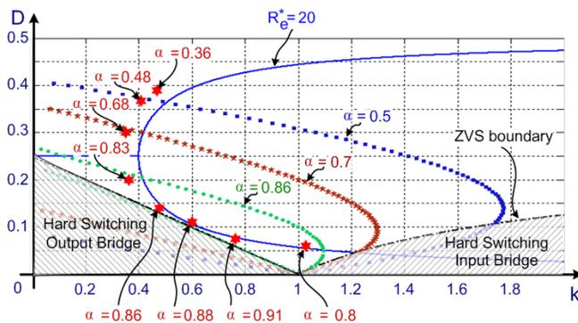
Figure 8: Generic model: Theoretical (line and dots) vs. experimental results (Red stars).
