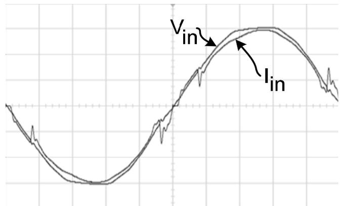
Figure 10: Typical waveforms. Voltage: 50V/Div; Current: 500ma/Div; Time: 2ms/Div;
