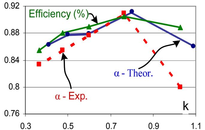
Figure 9: Theoretical and measured conduction losses index ( $\alpha$ ) and measured efficiency.
