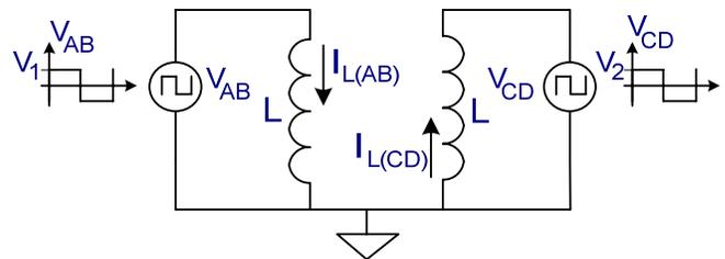
Figure 5: Simplified superposition inductor current analysis.
