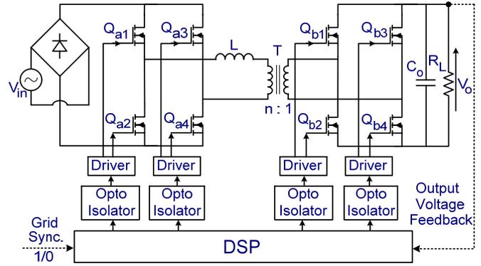
Figure 4: Proposed double bridge based APFC block diagram.
