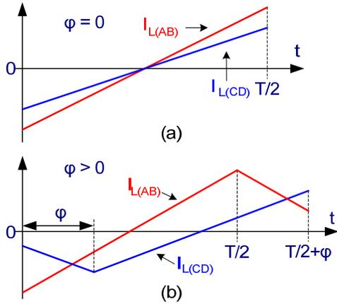
Fig. 6: Inductor current due to left ( $I_{L(CD)}$ ) and right ( $I_{L(AB)}$ ) bridges, (a)  $\varphi = 0^\circ$ , (b)  $\varphi > 0^\circ$ .
