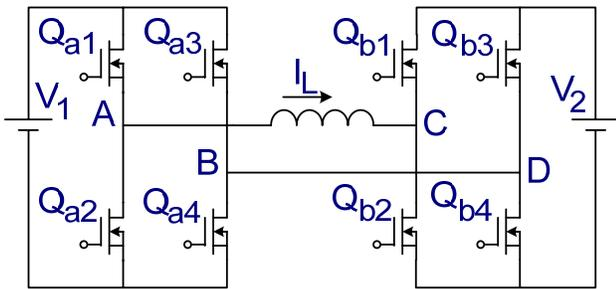
Figure 2: Double bridge Gyrator-behaved topology.
