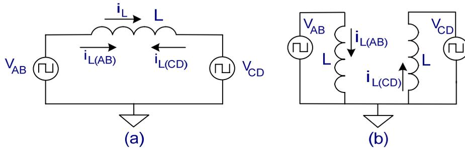
**Figure 3:** Inductor' current decomposition:
