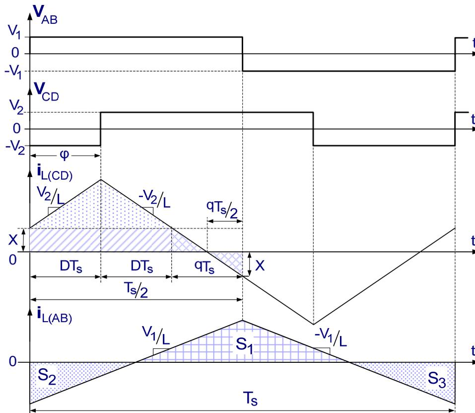
**Figure 4:** Contribution of the two bridges to the inductor current waveform.
