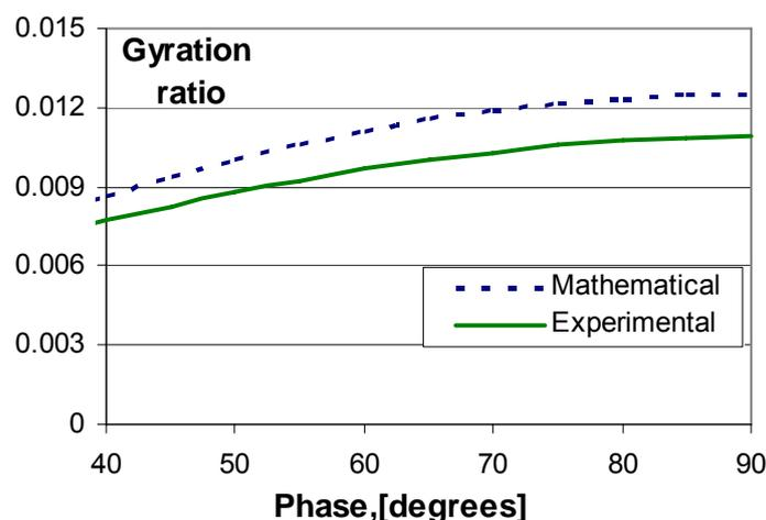
**Figure 12:** Gyration ratio: Dashed line – Mathematical computations, Solid line – Experimental results.
