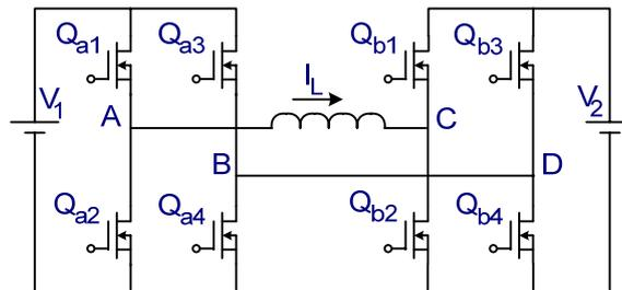
Figure 2: Double bridge "AC inductor" circuit.
