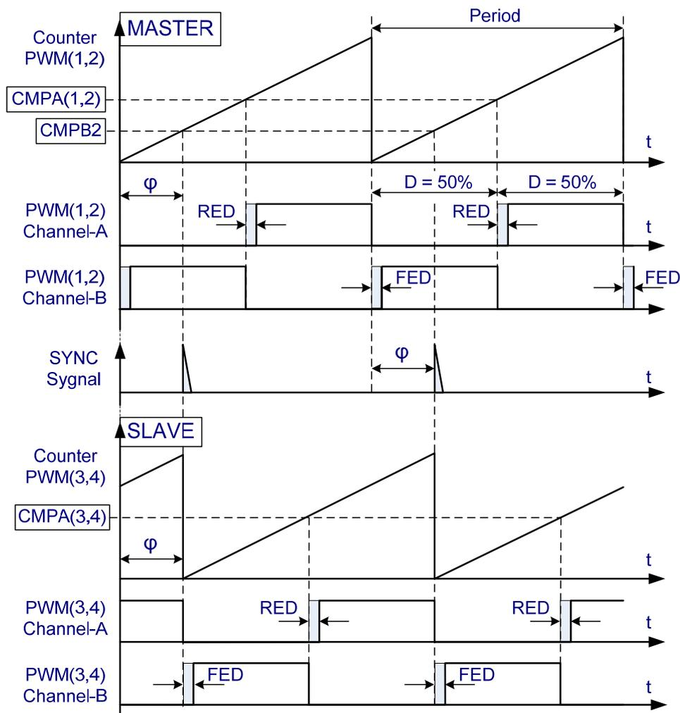
Figure 8: ePWM timing diagram. (CMPA/B(X) – Compare registers)
