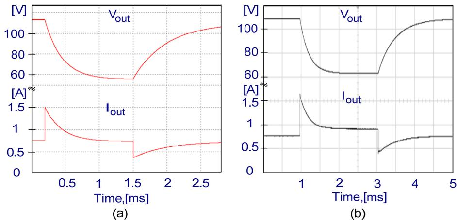
**Figure 11:** Load step up and step down between  $150\Omega$  and  $75\Omega$ : (a) Simulation, (b) Experimental.
