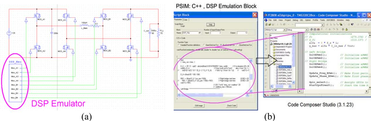
**Figure 6:** DSP emulation by a C++ block of "PSIM Professional 7.1.2.121: (a) PSIM simulation model. (b) The copy and paste process of the simulated C++ code into the code composer.
