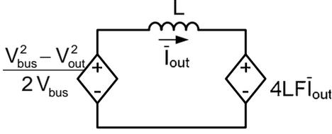
Fig. 8. Average large signal model of "AC inductor".
