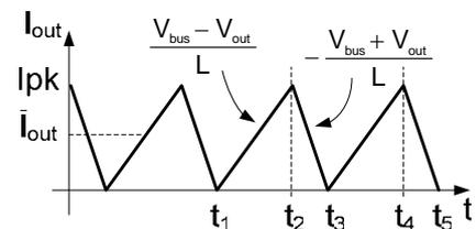
Fig. 4. Output current of an "AC inductor" converter.
