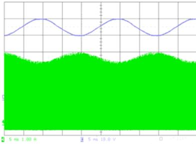
Fig. 13. Output current response to output voltage modulation. Upper trace: Modulating voltage 10V/div; Lower trace: Output current 1A/div; Horizontal scale: 5ms/div.
