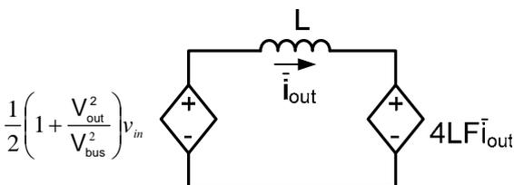
Fig. 9. Average small signal model of AC inductor charger linearized for a constant output voltage
