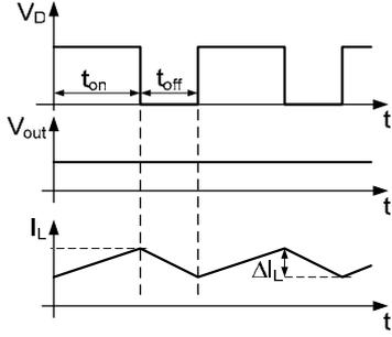
Fig. 2. Key waveforms of an ideal Buck converter.
