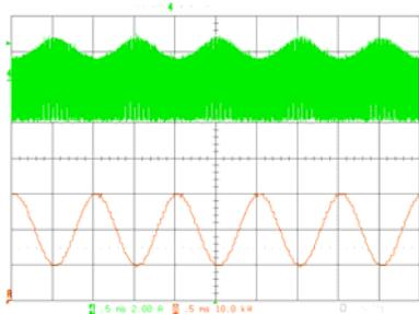
Fig. 14. Output current response to modulation of switching frequency. Upper trace: Output current 2A/div; Lower trace: Modulating frequency 10kHz/div; Horizontal scale: 0.5ms/div.
