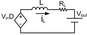
Fig. 5. Average model of a buck charger.
