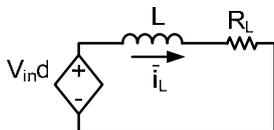
Fig. 6. A linearized average model of a DC inductor charger for constant input and output voltages.
