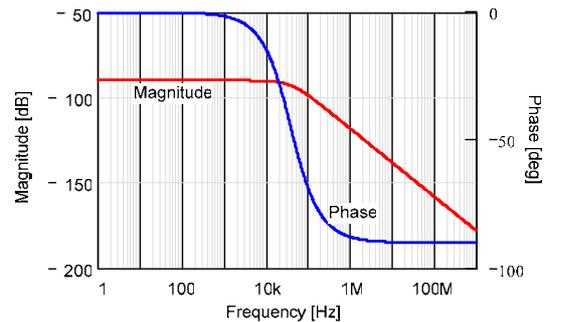
Fig. 11. Bode diagram of output current to switching frequency modulation transfer function (20).
