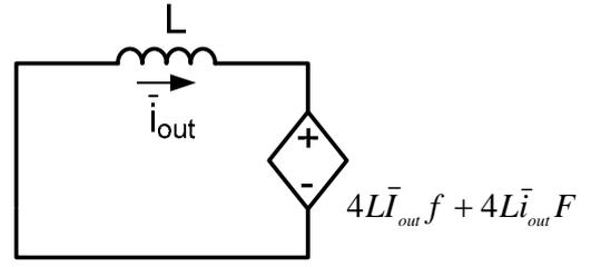
Fig. 10. Linearized average small signal model of AC inductor for small-signal injection in  $F, (f)$ .
