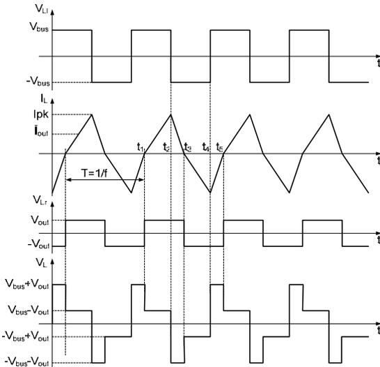
Fig. 3. Basic waveforms of the full bridge AC inductor converter.
