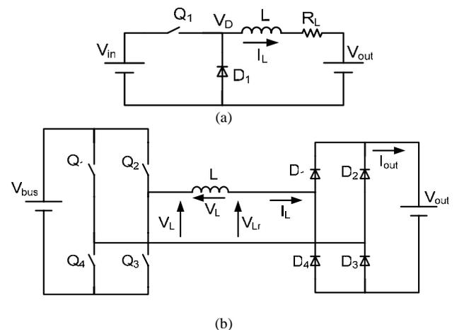
Fig. 1. Battery chargers. (a) Buck with DC inductor. (b) Full bridge with AC inductor.
