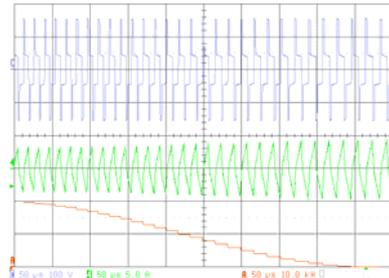
Fig. 15. Expanded view of AC inductor's key waveforms. Upper trace: Inductor's voltage: 100V/div. Middle Trace: Inductor's current 5A/div. Lower Trace: Switching frequency 10kHz/div (carrier frequency 62.5kHz). Horizontal scale: 50us/div
