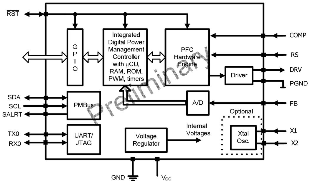
Figure 25: NGPD4102 Functional Block Diagram
