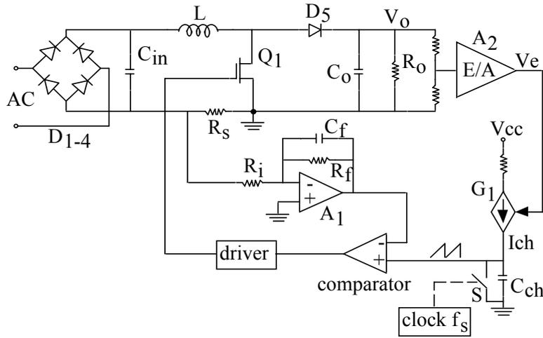
Figure 8: Realization of the multiplier action by a controllable slope.
