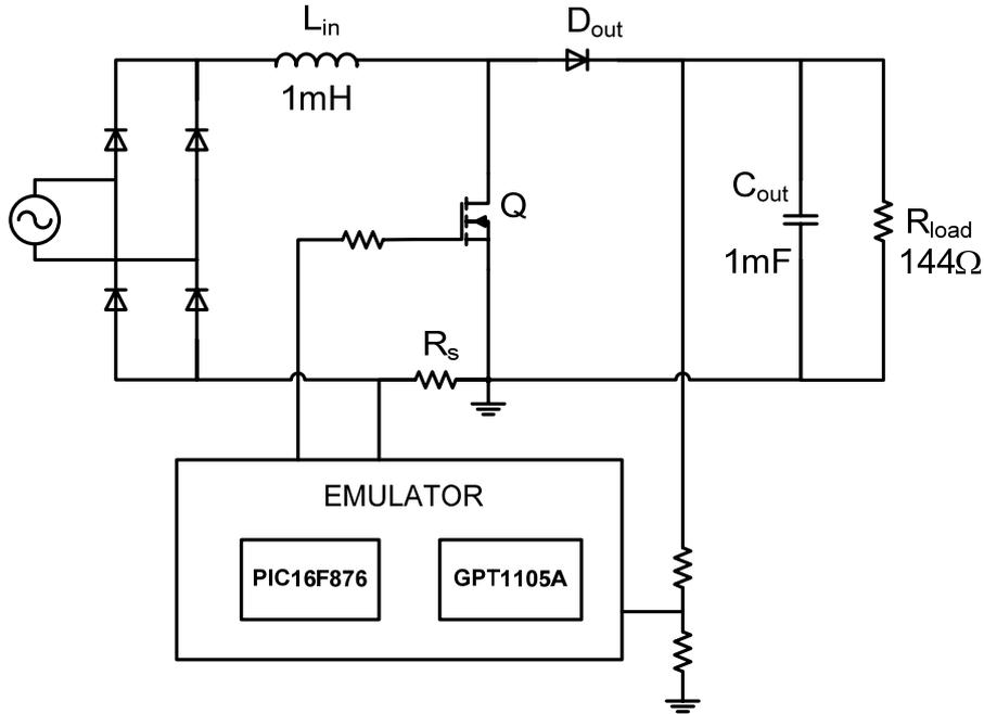
Figure 18: Experimental setup of 1kW PFC stage.
