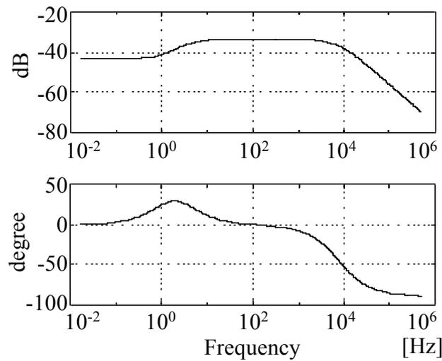
Figure 6: Transfer function of the current control loop.
