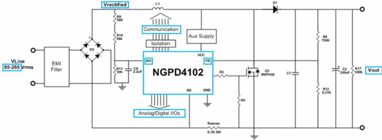
Figure 27: NGPD4102 Evaluation Board Functional Block Diagram
