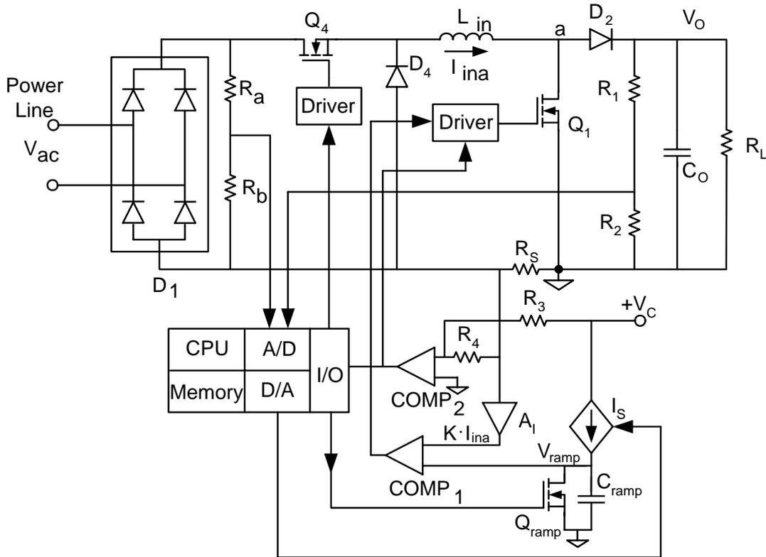
Figure 10: PWM-based implementation of inrush current
