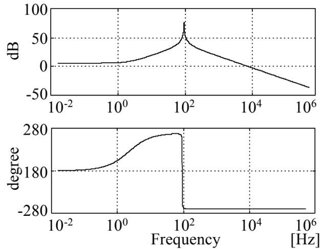
Figure 5: Loop gain of the current control loop.
