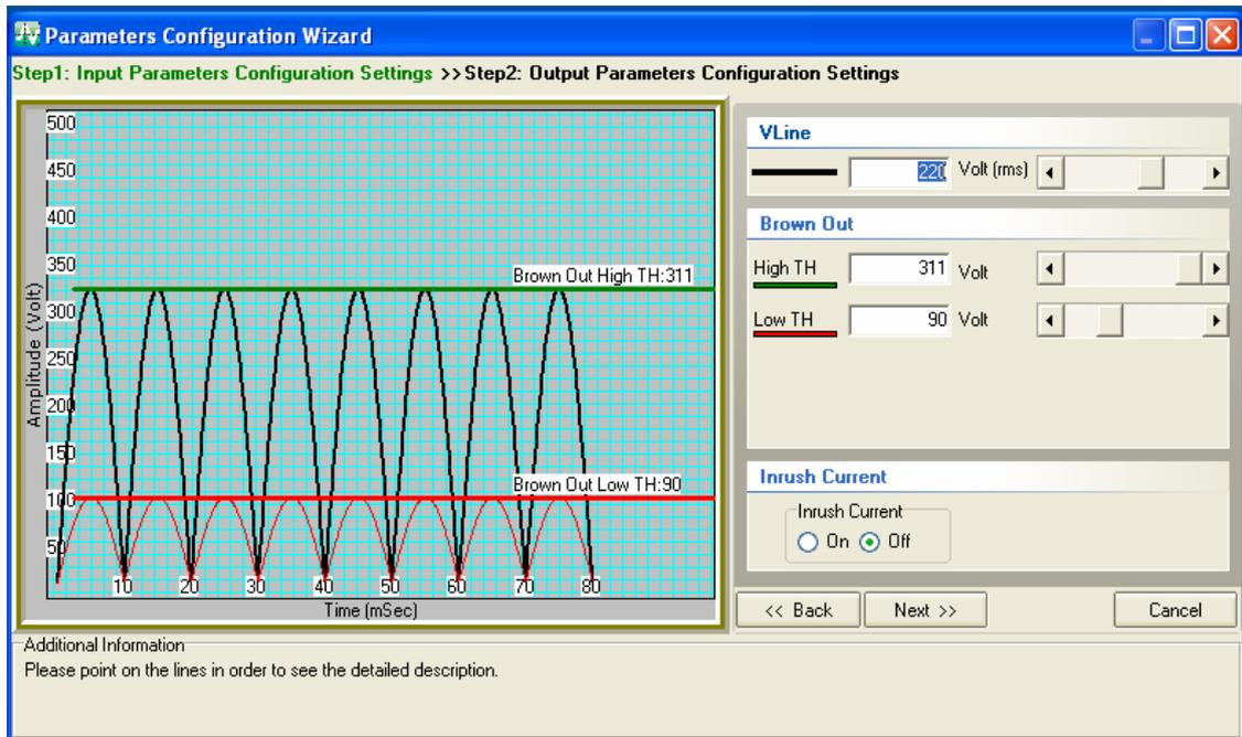
Figure 30: EVB GUI: Output parameters' settings
