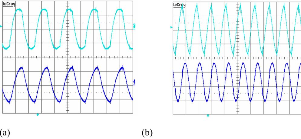
Figure 21: Lamps' voltage and current (one branch). (a) Full load ( $P_{in}=187W$ ). Upper trace: lamps' current 0.5A/div; Lower trace: lamps' voltage 200V/div; (b) Dimmed lamps ( $P_{in}=59W$ ). Upper trace: lamps' current 0.25A/div; Lower trace: lamps' voltage 200V/div. Horizontal scale: 20µs/div.
