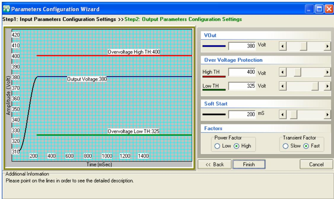
Figure 29: EVB GUI: Input parameters' settings
