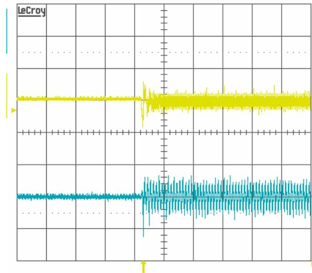
Figure 16: Load step.  $V_{in}=230V_{ac}$ ; Load=15W  $\rightarrow$  300W; Upper trace: output voltage – 20V/div; Lower trace: input current – 5A/div; Horizontal scale: 0.2s/div
