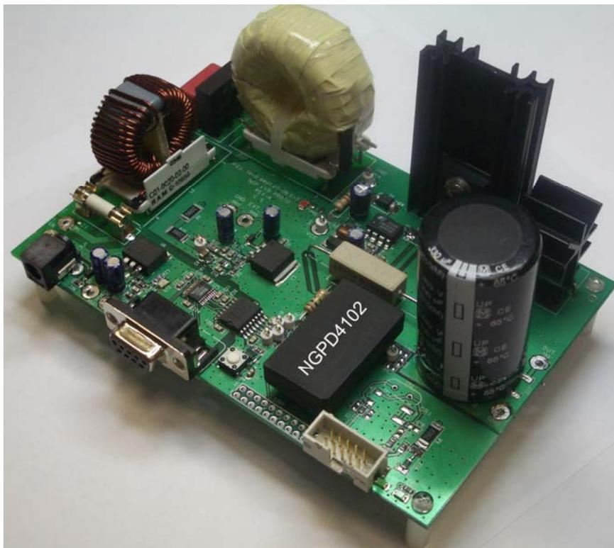
*Figure 28:* The NGPower EVB using the NGPD4102 emulator
