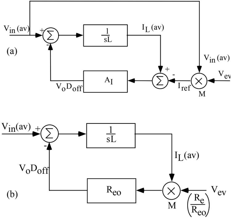
Figure 7: Block diagram of a conventional (a) and our solution for (b) power factor correction control.
