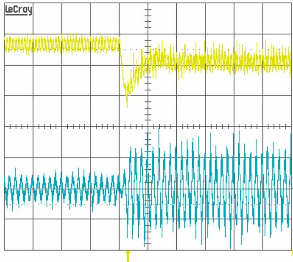
Figure 15: Input voltage step.  $P_{out}=300W$ ;  $V_{in}=265Vac \rightarrow 85Vac$ ; Upper trace: output voltage – 20V/div; Lower trace: input current – 5A/div; Horizontal scale: 0.1s/div
