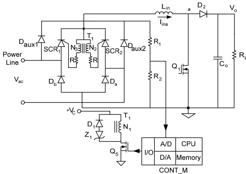
Figure 11: Thyristor-based implementation of inrush current
