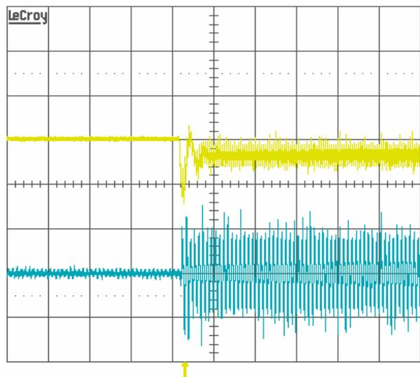
Figure 17: Load step.  $V_{in}=110V_{ac}$ ; Load=15W  $\rightarrow$  300W; Upper trace: output voltage – 20V/div; Lower trace: input current – 5A/div; Horizontal scale: 0.2s/div
