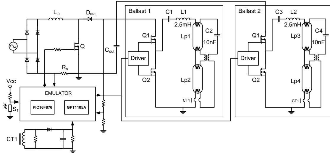
Figure 20: Experimental setup of digital PFC stage driving 2 lamp ballasts.
