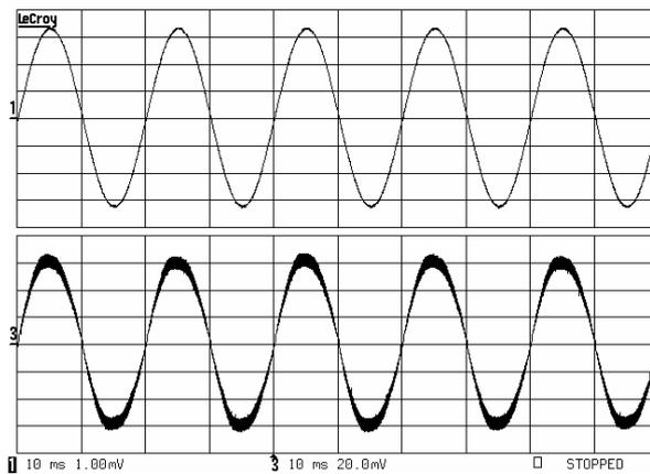
Figure 19: Input behavior of the system shown in Fig. 19. Upper trace: input current 2A/div. Lower trace: input voltage 230VAC. Horizontal scale: 10mS/div.  $V_{out}=385V$ .  $P_{in}=975W$
