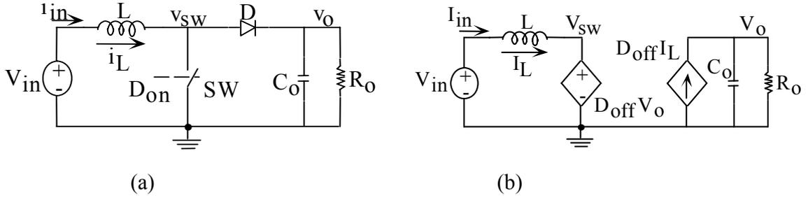
Figure 3: The Boost converter (a) and its behavioral average model (b) ([9, 10]). Assuming the circuit is stable (as will be shown below), this implies (Fig. 3b):
