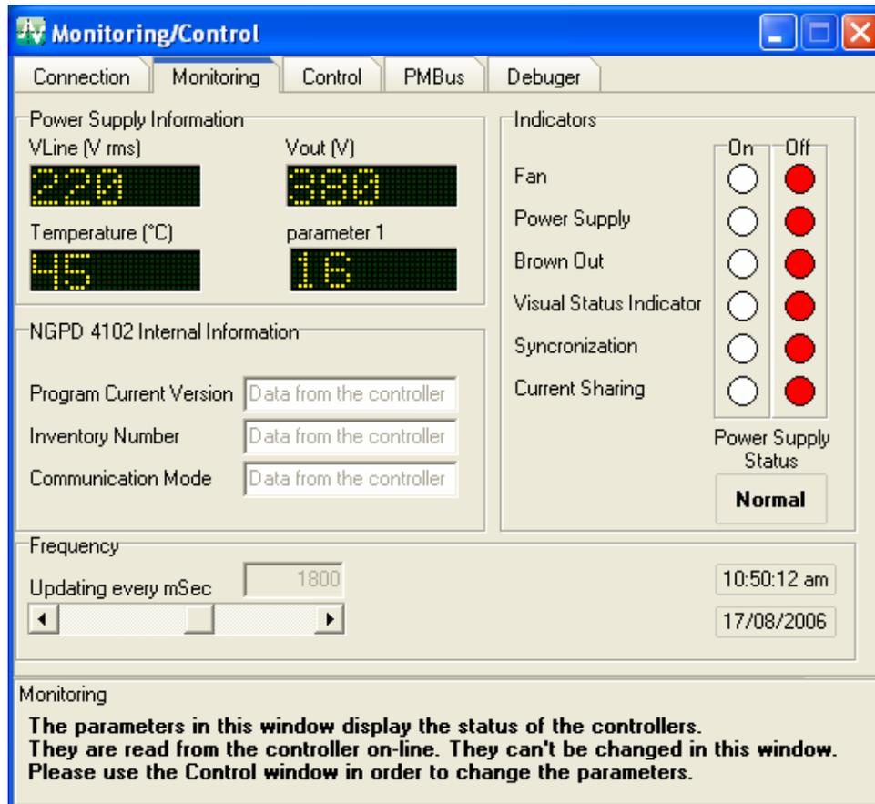
Figure 31: EVB GUI: Real-time parameter monitoring
