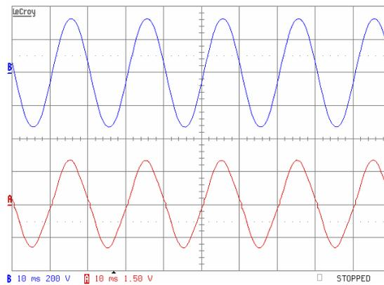
Figure 12: Input behavior.  $P_{out} \approx 300W$ . Upper trace: Input voltage 230Vrms. Lower trace: Input current 1.5A/div. Horizontal scale: 10ms/div.
