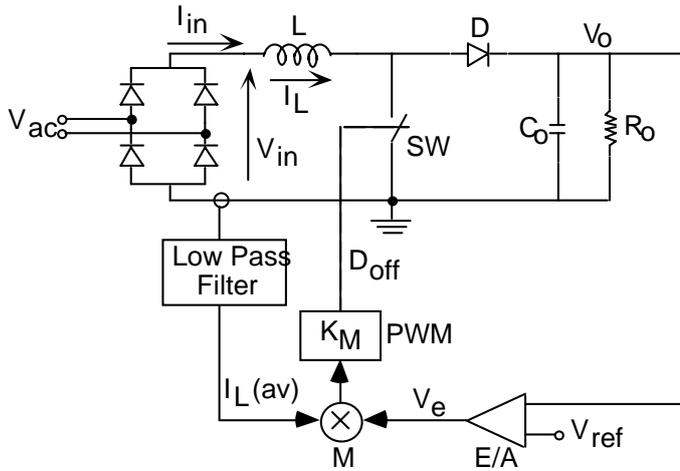
Figure 2: Implementation of an APFC control scheme with no sensing of input voltage.
