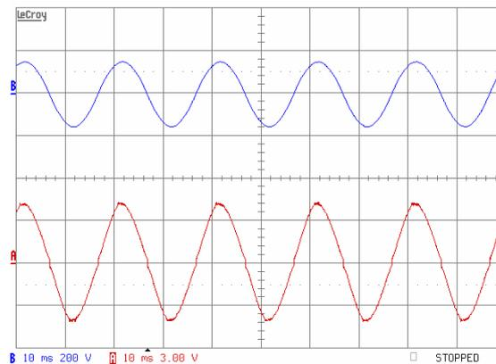
Figure 13: Input behavior.  $P_{out} \approx 300W$ . Upper trace: Input voltage 110Vrms. Lower trace: Input current 3A/div. Horizontal scale: 10ms/div.
