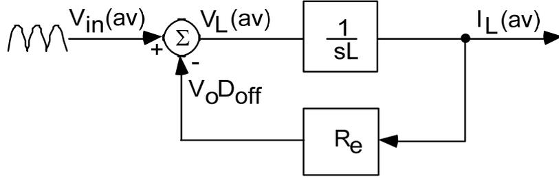
Figure 4: Simplified block diagram of current control loop.
