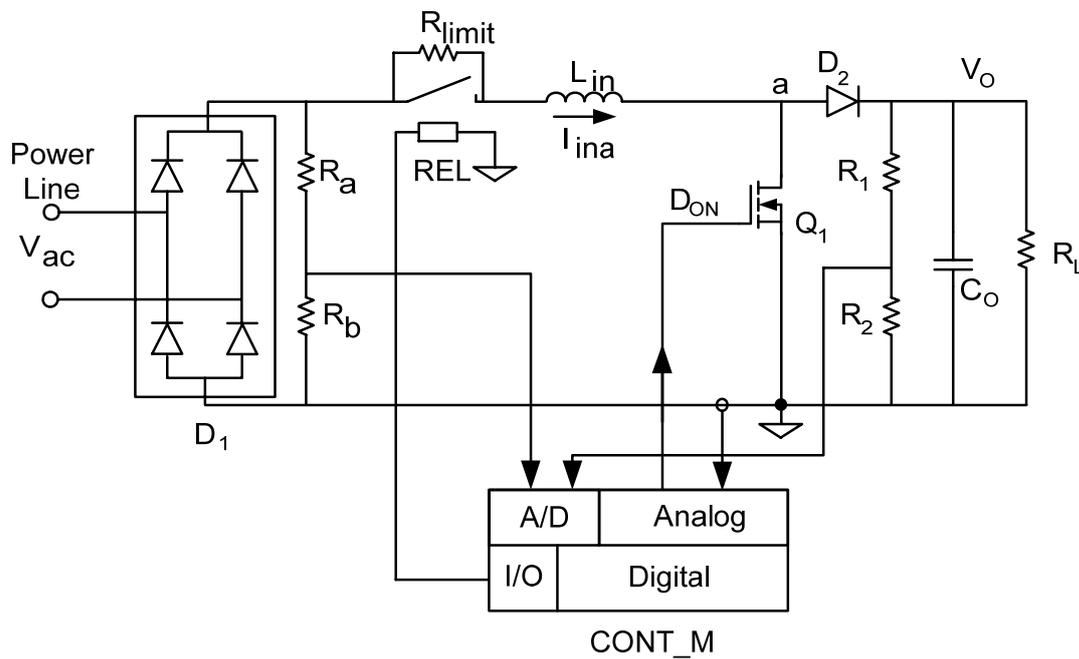
Figure 9: Relay-based implementation of inrush current
