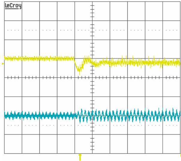
Figure 14: Input voltage step.  $P_{out}=50W$ ;  $V_{in}=265Vac \rightarrow 85Vac$ ; Upper trace: output voltage – 10V/div; Lower trace: input current – 5A/div; Horizontal scale: 0.1s/div
