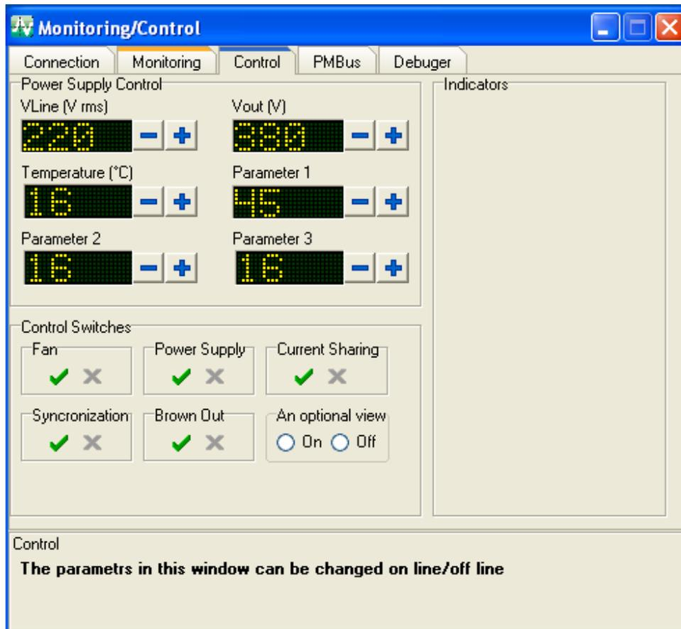
Figure 32: EVB GUI: Real-time parameter control
