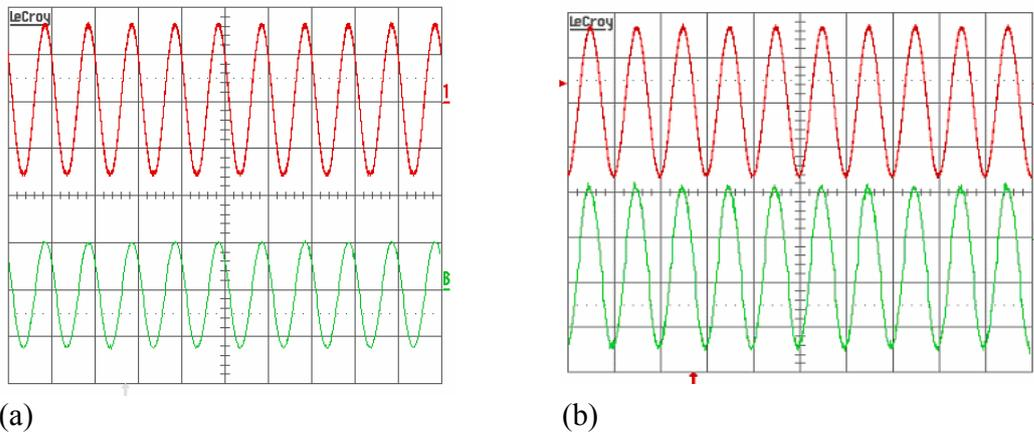
Figure 22: Input behavior of the front-end of Fig. 21. (a) Full load ( $P_{in}=187W$ ). Upper trace: input voltage (230Vac); lower trace: input current 1A/div. (b) Dimmed lamps ( $P_{in}=59W$ ). Upper trace: input voltage (230Vac); lower trace: input current 0.2A/div. Horizontal scale 10ms/div.
