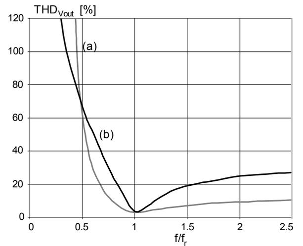
Figure 6. Total Harmonic Distortion of output voltage as a function of the deviation from the resonant frequency. (a) CFPPRI-US (numerical calculation). (b) The basic CFPPRI (SPICE simulation).
