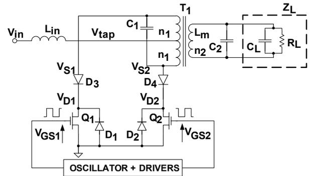
Figure 3. The CFPPRI with diodes in series to the power switches.
