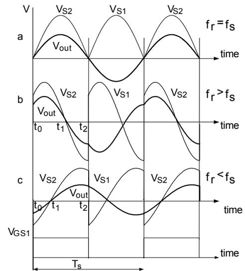
Figure 4. Gate voltage ( $V_{GS1}$ ), switch voltages ( $V_S$ ) and output voltage ( $V_{out}$ ) when the gate-drive frequency matches the resonant frequency (a) and when it is lower (b) or higher (c) than the resonant frequency.
