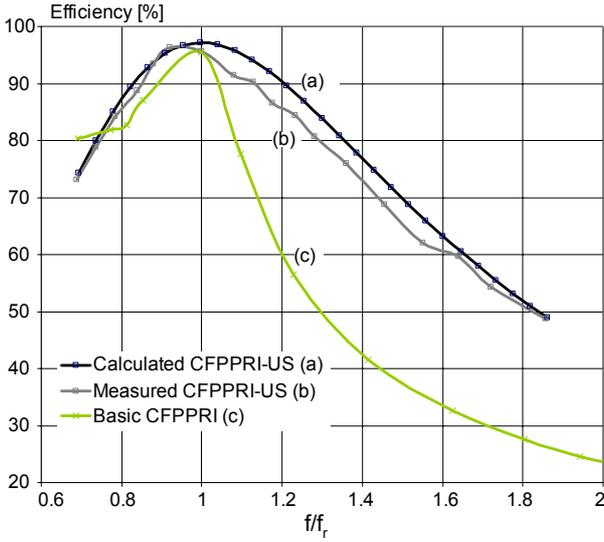
Figure 7. Efficiency as a function of the deviation from resonant frequency. (a) Calculated efficiency of the CFPPRI-US. (b) Measured efficiency of the CFPPRI-US. (c) Measured efficiency of the basic CFPPRI topology.
