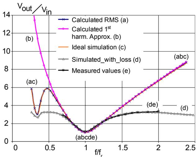
Figure 9. Measured, simulated and calculated output gain of the CFPPRI-US as a function of the deviation from the resonant frequency.
