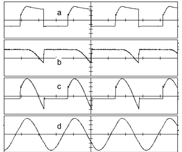
Figure 8. Experimental results. The inverter is loaded by a rotary piezoelectric motor (below resonance operation,  $f/f_r = 0.65$ ). (a)  $V_{D1}$  (10V/div). (b)  $V_{D3}$  (20V/div). (c)  $V_{D3}+V_{D1}$  (10V/div) and (d) output voltage (50V/div). Horizontal scale (5 $\mu$ s/div).
