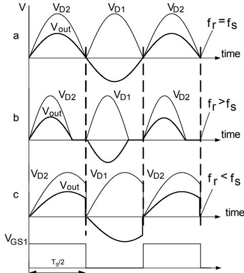
Figure 2. Gate voltage ( $V_{GS1}$ ), drain voltages ( $V_D$ ) and output voltage ( $V_{out}$ ) when the gate-drive frequency matches the resonant frequency (a) and when it is lower (b) or higher (c) than the resonant frequency.
