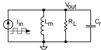
Figure 5. Simplified CFPPRI circuit.
