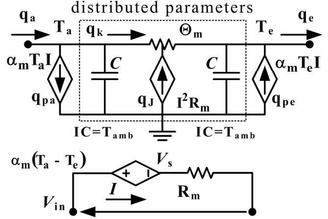
Fig. 2. The equivalent circuit of the TEC. The scheme is based on a Cauer-type network for describing heat transfer in a solid with internal heat sources ( $q_j$ ).  $q_{pa}$  and  $q_{pe}$  (Peltier cooling and heating). The  $V_s$  voltage source describes Seebeck power generation.  $IC$  is the initial temperature of the device,  $T_{amb}$ .
