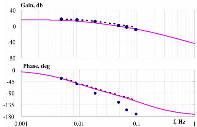
Fig. 7. Transfer function of the system of Fig. 6. Input variable is the input voltage and output is the temperature difference between the aluminum plates on both sides of the TEC. Dashed line is the result of cycle-by-cycle transient simulation of the system with sine input voltage (amplitude 1.3 V); Solid line is the small-signal (ac) simulation result, and points are data of the experimental measurements.
