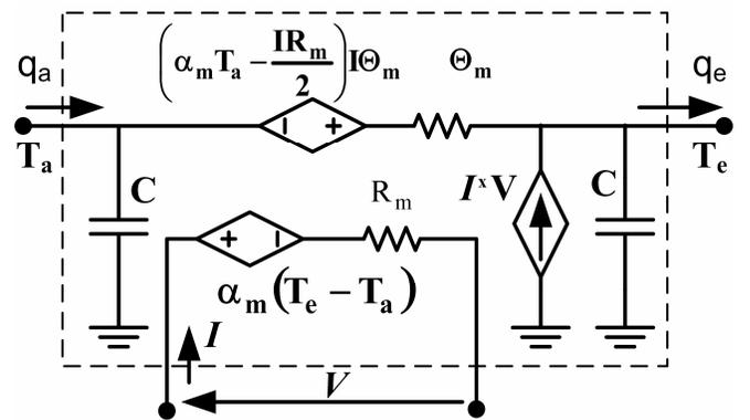
Fig. 3. Modified proposed equivalent circuit of a thermoelectric module.
