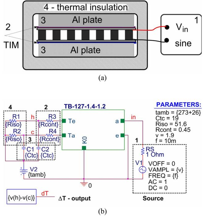
Fig. 6. Measurement of the small-signal transfer function of the system: TEC sandwiched between two massive aluminum plates with built-in thermocouples. (a) Experimental setup. (b) PSPICE/OrCAD simulation scheme. The model of the TEC is the one shown in Fig. 3 with parameters  $\alpha_m=0.053$  V/K,  $R_m=1.6$   $\Omega$ ,  $\Theta_m=1.5$  K/W calculated above, 1: sine voltage source, 2: thermal interface material (TIM), 3: aluminum plates.
