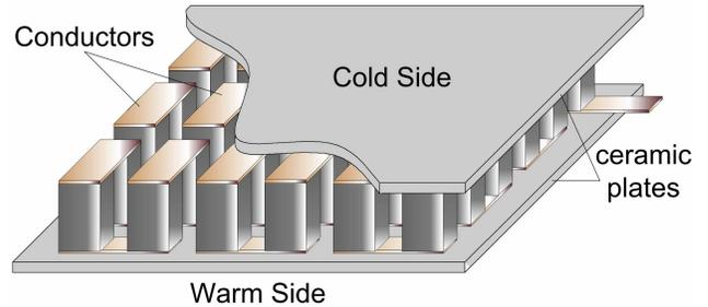
Fig. 1 Single-stage thermoelectric module construction
