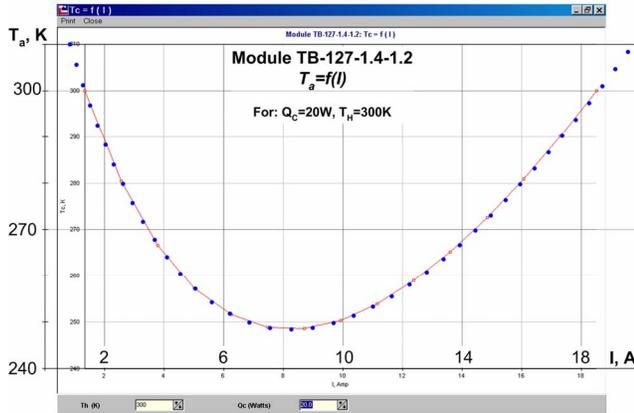
Fig. 4. Performance plot of TEM: TB-127-1.4-1.2. Temperature of the a-side (cold) vs. current under conditions:  $T_h=300$ , cooling power 20W. The dashed line is the simulation result obtained by the proposed model; the solid line is the performance plot published by the manufacturer.
