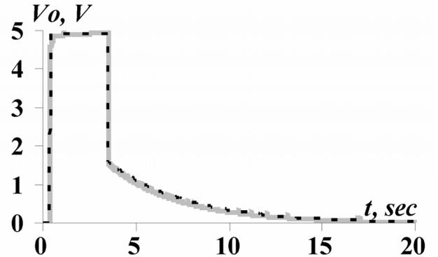
Fig. 5. Time response of the TEC. The gray thick line shows the result of the experiment on the physical module. The black dashed line is the result of the computer simulation using PSPICE (black line).
