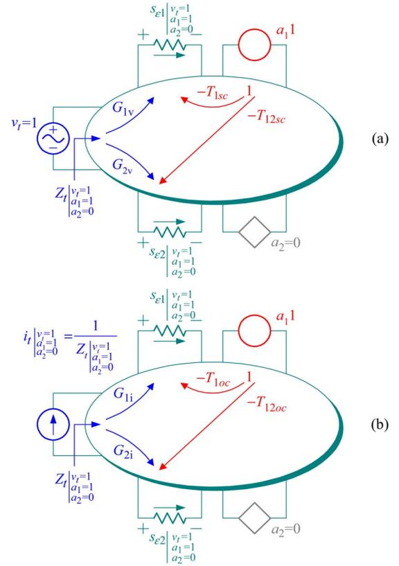
Fig. 3. Generic feedback network with two dependent sources, where  $v_t = 1$ ,  $s_{\epsilon 1} = 1$ , and  $s_{\epsilon 2} = 0$ .
