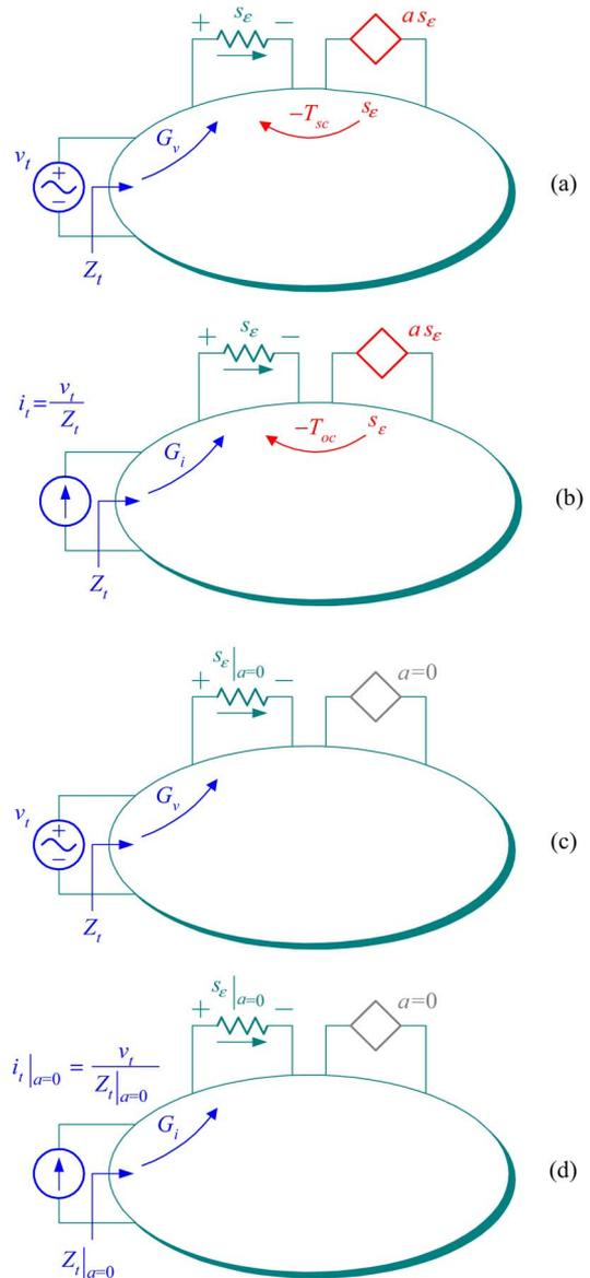
Fig. 1. Finding the impedance seen by a test source connected to arbitrary terminals of a generic feedback network with a single dependent source.
