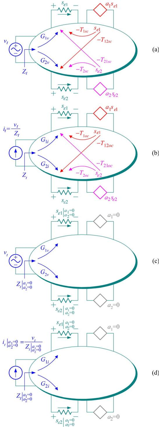
Fig. 2. Finding the impedance seen by a test source connected to arbitrary terminals of a generic feedback network with two dependent sources.
