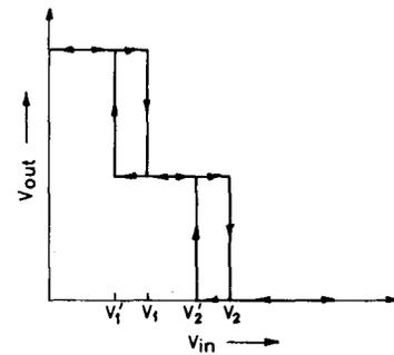
Fig. 1. Transfer characteristics of a ternary Schmitt trigger.
