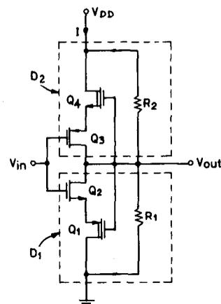
Fig. 4. Circuit schematic of the ternary Schmitt trigger.
