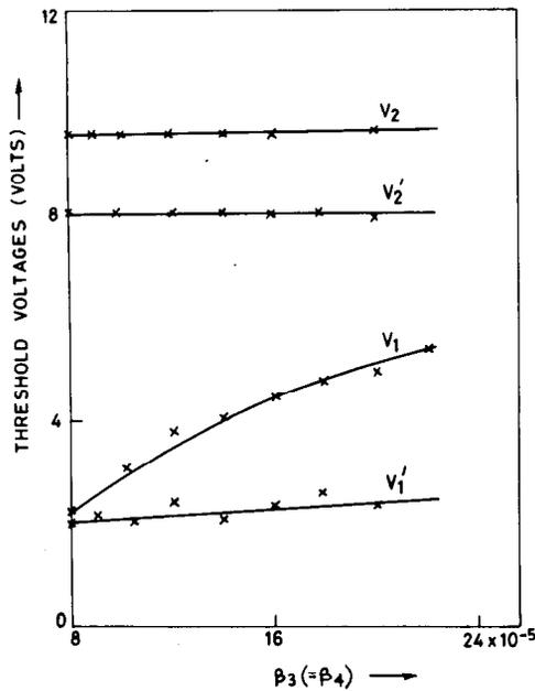
Fig. 7. Dependence of the threshold voltages on  $\beta_3$  and  $\beta_4$ .
