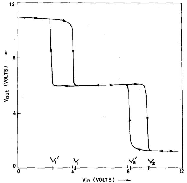
Fig. 6. Simulated transfer characteristics of the ternary Schmitt trigger.
