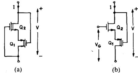
Fig. 2. (a) Lambda diode. (b) Lambda transistor.
