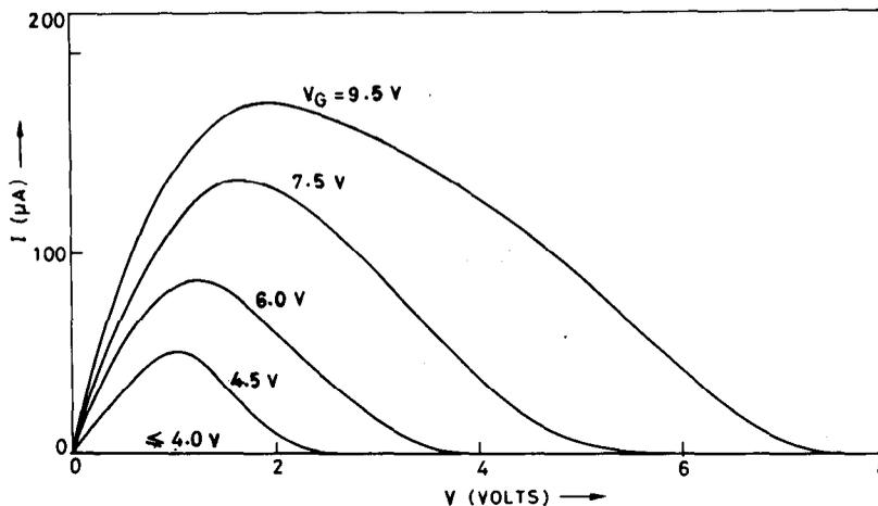
Fig. 3. Simulated  $V-I$  characteristics of the lambda transistor.
