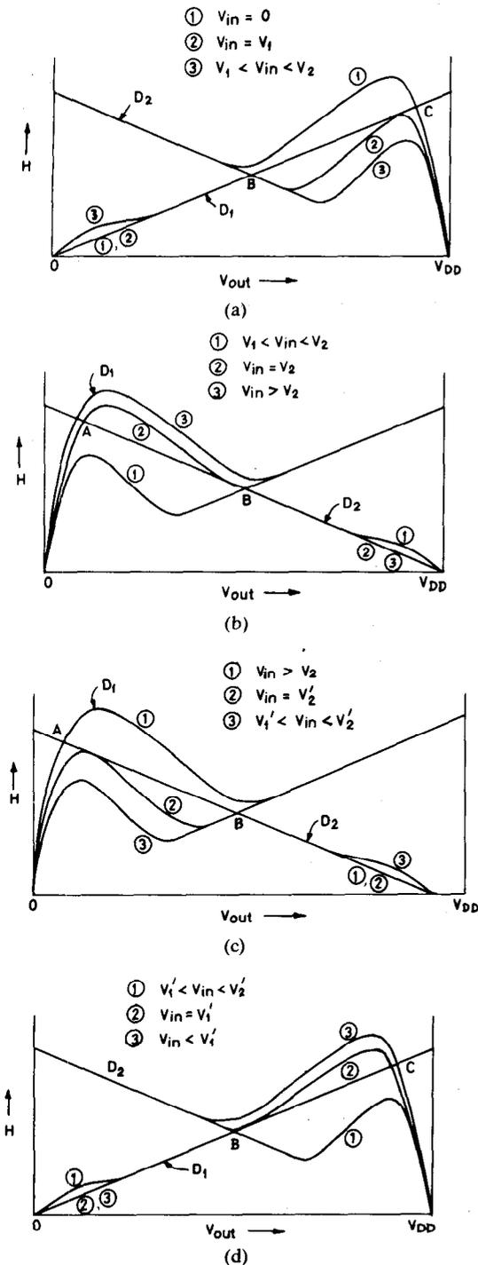
Fig. 5.  $V$ - $I$  characteristics of  $D_1$  and  $D_2$  under various input conditions. (a)  $V_{IN}$  increasing, in the vicinity of  $V_1$ . (b)  $V_{IN}$  increasing, in the vicinity of  $V_2$ . (c)  $V_{IN}$  decreasing, in the vicinity of  $V_2'$ . (d)  $V_{IN}$  decreasing, in the vicinity of  $V_1'$ .
