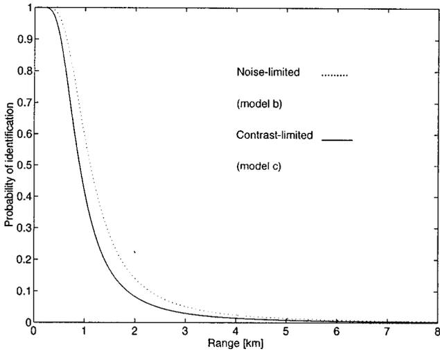
**Fig. 19** Probability of identification versus range for the midnight experiment. Range is 2.3 km.
