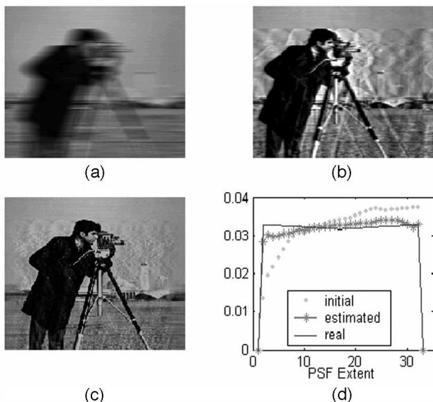
Fig. 3. (a) Cameraman image degraded by a 33-pixel portion of a low-frequency sinusoidal motion blur; (b) image restored by a direct method; (c) image restored by the proposed direct-iterative RL method; and (d) real, initial, and final estimated PSFs.
