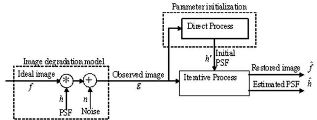
Fig. 2. Block diagram of the degradation and the combined direct-iterative blind deconvolution processes.
