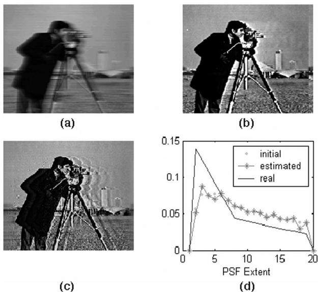
Fig. 6. Same as Fig. 3, but for another motion type obtained by using a different portion of a low-frequency sinusoidal blur with a 20-pixel extent and with a restoration using the EM iterative method.
