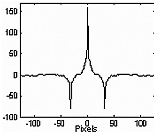
Fig. 4. Average ACF that produces the initial PSF estimation of the direct method from the blurred image of Fig. 3(a). The distance between a global minimum and the center of the ACF (33 pixels in this case) is the blur extent estimation of the direct method.
