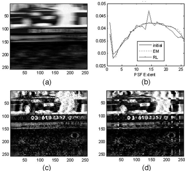
Fig. 7. (a) Real-motion-blurred image taken from a moving car,<sup>6</sup> (b) comparison of PSFs estimated by the direct-only method and by the proposed direct-iterative EM and RL methods for a blur extent estimated as 26 pixels, (c) image restored by the direct-iterative EM method, and (d) image restored by the direct-iterative RL method.
