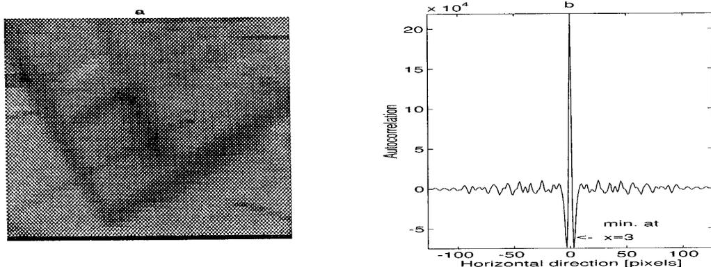
FIG. 8. (a) The image *phone* mechanically blurred horizontally by low frequency vibrations; (b) a 3-pixel blur extent was identified by a clear minimum in the identification function.
