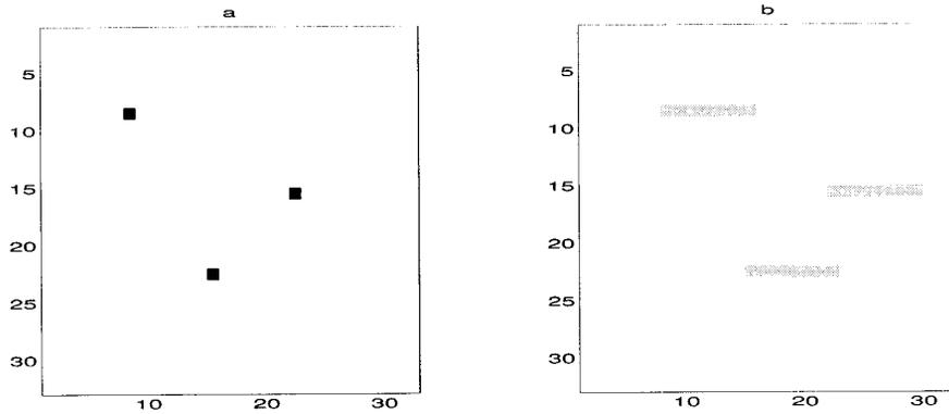
FIG. 1. (a) A 3-pixel image; (b) The blurred image using an 8-pixel square function.
