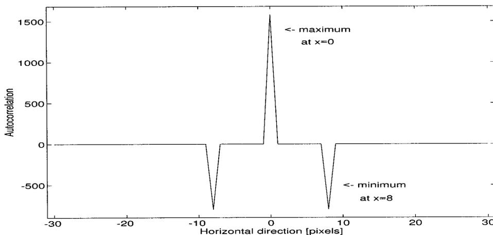
FIG. 3. The ACF of row 15 in the image derivative of Fig. 2. The blur extent (8 pixels) is equal to the location of the minimum of the function relative to the center.
