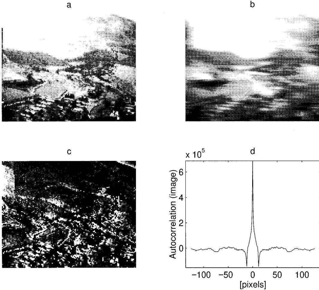
FIG. 6. Implementation for a real image. (a) The original *valley* image; (b) image blurred by horizontal accelerated motion function forming 12-pixel blur extent with 1.07 relative homogeneity of the PSF, and an additive zero mean normally distributed random noise causing 40 dB SNR; (c) the horizontal image derivative; (d) the average of the ACFs of the image derivative lines.
