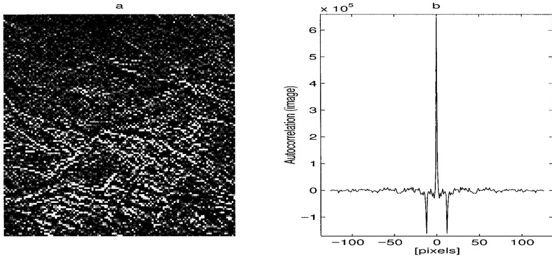
FIG. 7. (a) The horizontal derivative of the vertical derivative of the blurred valley image; (b) the average of the ACFs of the image derivative lines of (a).
