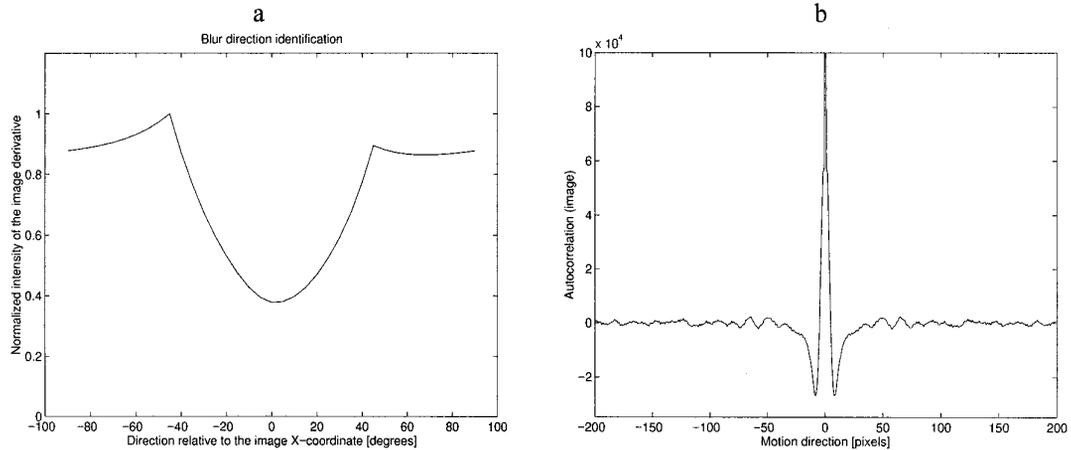
FIG. 14. (a) Zero degrees motion direction is identified in the direction identification function; (b) 8 pixels blur extent is identified by the ACF of the blurred image derivative.
