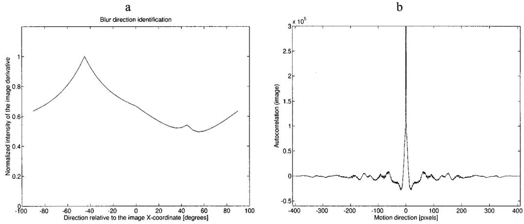
FIG. 11. (a) The motion direction ( $55^\circ$ ) is indicated by the location of the minimum in the motion direction identification function; (b) 18 pixels blur extent is identified by the ACF of the blurred image derivative.
