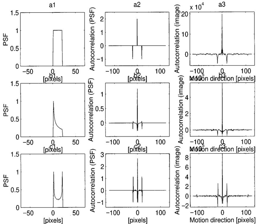
FIG. 16. Identification results for different motion types implemented on valley image. (a1, b1, c1) the blurring PSFs; (a2, b2, c2) the ACFs of the PSFs; (a3, b3, c3) the average of the ACFs of the blurred image derivative lines.
