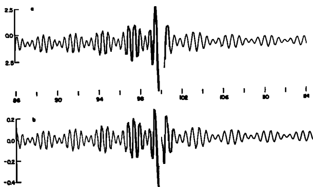
Fig. 3. (a) absolute value of total field, and (b) phase of total field both normalized with respect to the field of the object at rest. The velocity is \beta = 0.1 . The center kvt = 100 is the retardation time of the observer with respect to the origin x = 0 .
