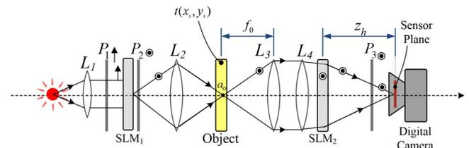
**Fig. 2.** Optical configuration of the SI-imaging based on the same optical arrangement as that of the SI-FINCH.
