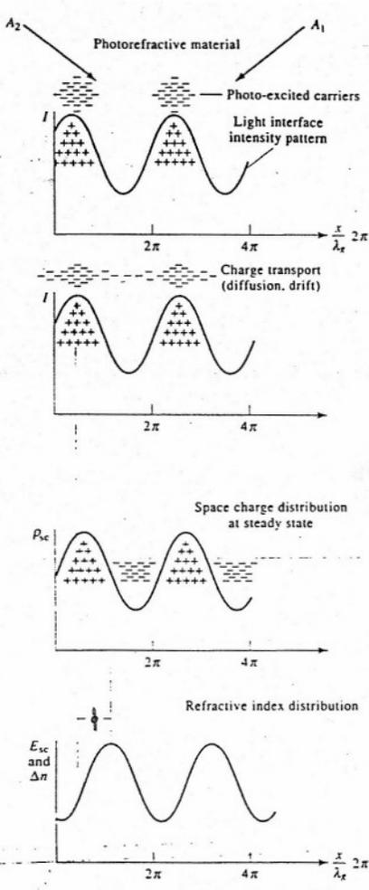
Figure 18-2 The photorefractive mechanism. Two coherent light beams intersect in an electrooptic crystal, forming an interference pattern. Electrons are excited where the intensity is large and migrate to regions of low intensity. The electric field associated with the resultant space charge operates through the electrooptic effect to produce a refractive index grating.  $\phi$  is the phase shift (in radians) between the light interference pattern and the index grating.
