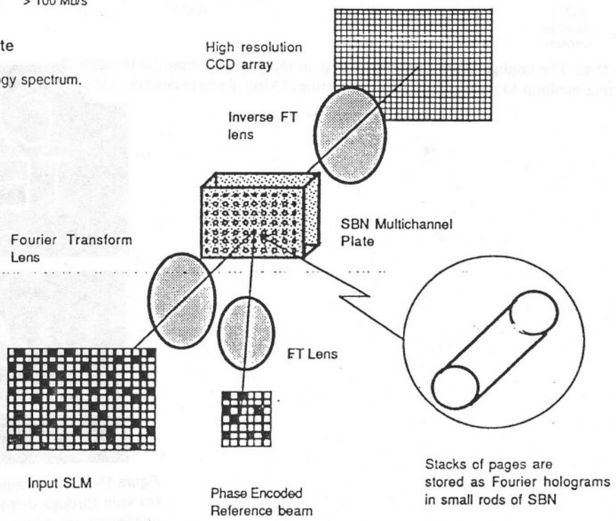
Figure 1 Schematic of a high-density, high-bandwidth data storage architecture.
