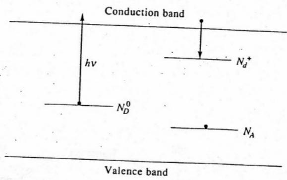
Figure 18-3 The deep impurity levels involved in the charge migration and trapping of a photorefractive crystal.
