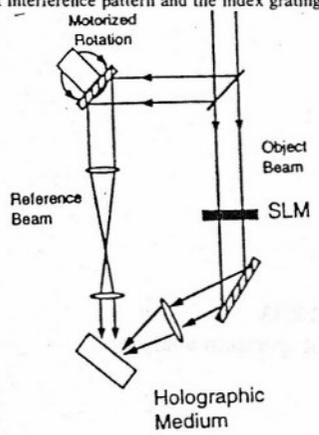
Fig. 7 Simplified angularly multiplexed storage system.
