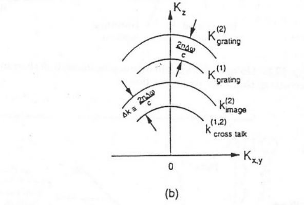
Figure 1-2. K space diagrams for volume holography using (a) angle-multiplexing scheme, (b) orthogonal multiplexing scheme
