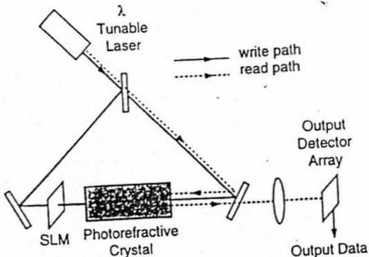
Fig. 9 Simplified wavelength multiplexed storage system.
